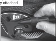
7. To test the connection, slowly open the cylinder valve and pressurize the regulator. Lift up on the lever and listen for the flow of air into the BC bladder.
