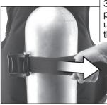
While holding the cylinder secure, pull the free end of the cylinder band until there is a very tight fit between the pack and the cylinder.
