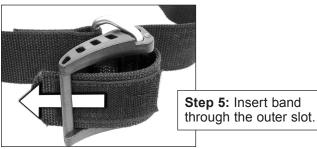
**NOTE:** This final threading step is done when the BC is secured to the cylinder (refer to step 4, p. 7). Close the buckle halfway to prevent the webbing from slipping and thread the free end of the band through the open slot in the end of the buckle.
