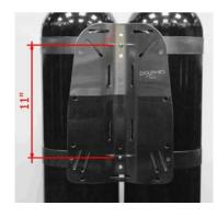
7) Repeat step 5 & 6 with the bottom tank band. Please note the distance from the top band should be 11" (centre to centre). It is easier using a back plate to measure.
