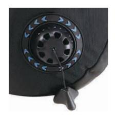
Fach air cell discussed previously is equipped at least 1 rapid exhaust valve which automatically releases excess gas when the pressure inside the bladder is 0.17kg/cm<sup>2</sup> (2.4psi) greater than the ambience to protect the bladder from bursting.
