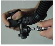
4) Open the tank valve SLOWLY. Check for any air leakage and proper power inflator function before using the air cell.
