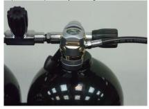
3) Pull back the quick disconnect sleeve in the female end of the low pressure BC hose and connect
