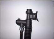
Inflate the BC by pressing the power inflation button. Use short bursts to control the amount of air entering the BC. The oral inflation mouthpiece allows for oral inflation by exhaling into the mouth piece while completely depressing the deflate button.
