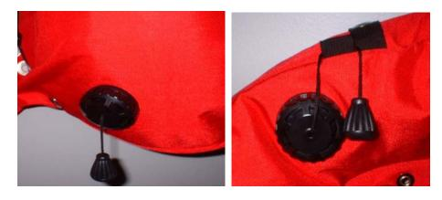
Pull dumps should be inspected regularly by fully inflating the BC to insure they vent properly. Also, be sure to thoroughly rinse them after each dive to prevent debris from becoming trapped in the seal causing air to leak from the BC.
