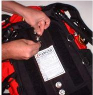
Install the flat washer first (against the backplate or harness) then the split lock washer. Thread the wingnuts onto the bolts and tighten securely by hand. Next install two nylon cam bands through the slots on the Single Tank Adaptor. Weave the webbing of the tank band through the cam buckle using the weave outlined on page 34. Remember, all nylon webbing stretches when wet so be sure to soak the nylon tank bands in water before tightening.
