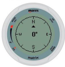
The number shown in the middle of the compass rose represents the bearing, between 0 (North) and 359.
