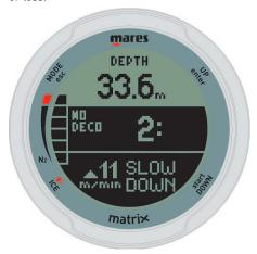
If the ascent rate exceeds 12m/min / 40ft/min at a depth below 12m / 40ft, the message on the screen changes to **TOO FAST**. If a speed in excess of 12m/min / 40ft/min is maintained for two thirds or more of the depth at which the alarm was first triggered, Matrix considers it a dive violation and the display will show  $\triangle$ .
