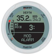
The alarm persists until the diver has ascended enough for the  $ppO_2$  to return within the set limit. While the alarm is active, the compass can only be called up for 8 seconds, after which the default display with the alarm message is shown again.
