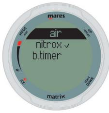
Use the buttons on the right side to highlight your choice, then press and hold the top right button to activate it.  $\operatorname{air}$  is the equivalent of setting  $\operatorname{nitrox}$  to 21% and a  $\operatorname{ppO}_2$ max of 1.4bar, but simplifies the display a bit by not showing the CNS (its value however is calculated in the background and if needed the 75% warning and the 100% alarm are triggered).
