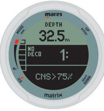
When the oxygen toxicity level approaches 100%, the alarm message CNS > 100% appears. The alarm message and the audible signal are repeated for 5 seconds in one-minute intervals after the first occurrence and for as long as the value of CNS stays at or above 100%. Consider terminating the dive immediately!
