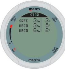
The stop summary table has an 8-second time-out, after which the screen automatically reverts to the default computer display. You can exit the stop summary table before the 8 seconds are passed by pressing the top left button
