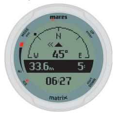
By pressing and holding the bottom right button you activate the stop watch. This can be helpful when timing yourself on the leg of a navigation course. Every time you press and hold the bottom right button, the stop watch restarts from 00:00. If you exit the compass the stop watch keeps running in the background.
