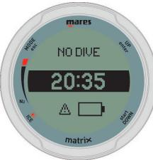
The exact level of the battery charge can be viewed at the bottom of the display by scrolling through the information using the bottom right button (see section 1.4).
