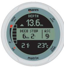
DEEP stops are generated as you approach the no deco limit. You can either have one 2-minute stop or two 1-minute stops. DEEP stops are NOT mandatory.
