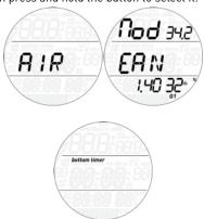
**AIR** is the equivalent of setting **EAN** to 21% and a  $ppO_2max$  of 1.4bar, but simplifies the display a bit by not showing the CNS (its value however is calculated in the background and if needed the 75% warning and the 100% alarm are triggered).
