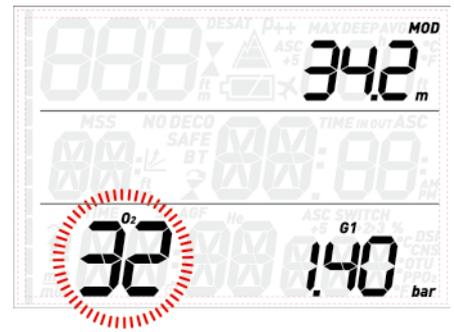
Once inside this menu, press the **UP** or **DOWN** button to change the O<sub>2</sub>% and observe how this affects the maximum operating depth (MOD). Then press the **ENTER** button to move on to the ppO<sub>2</sub>max and use the **UP** or **DOWN** button to change the value, again noticing how this affects the MOD. Press the **ENTER** button again to save the setting.
