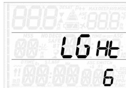
Quad has a backlight which can be activated in case of low ambient light. The backlight is activated by pressing and holding either of the upper buttons. During a dive, the backlight will stay on for the duration defined in this menu. You can choose between 1 and 10 seconds or you can set it to **on**. If you set it to **on**, the backlight will remain on until you press and hold either of the upper buttons again.
