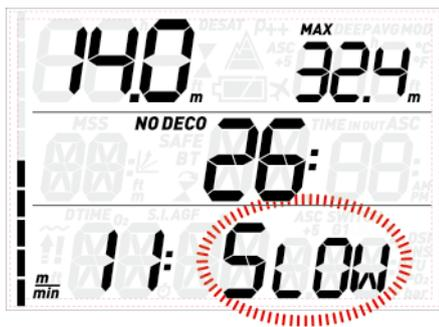
If the ascent rate exceeds 12m/min / 40ft/min at a depth below 12m / 40ft, blinks as well. If a speed in excess of 12m/min / 40ft/min is maintained for two thirds or more of the depth at which the alarm was first triggered, Quad considers it a dive violation and the display will show the steady .
