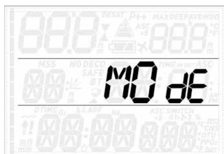
Here you can define the type of gas you will be breathing during the dive (air or enriched air nitrox, including multigas). You can also set Quad to bottom timer, in which case Quad will show only time, depth and temperature: it will not carry out any decompression calculation and it will not show any warnings and alarms.
