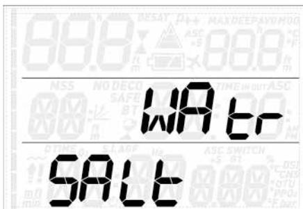
You can set the computer for **FRESH** water, **SALT** water or **EN13319** calibration, depending
