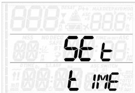
This menu allows you to set the time and date. Press the **ENTER** button and **24h** or **AMPM** will start to blink. Press the **UP** or **DOWN** button to switch between the two and/or press the **ENTER** button to confirm and move on to set the hour, the minutes and the date.
