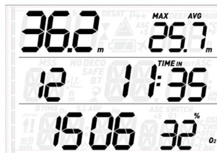
Press **ENTER** to view the next page of the dive log, which shows the surface interval prior to the dive alternating with the dive time and **CNS** (alternating between start and end value) in the bottom row. In case more than one gas was used in the dive, information about **G2** and **G3** if applicable is shown alternating with G1 on the first page.
