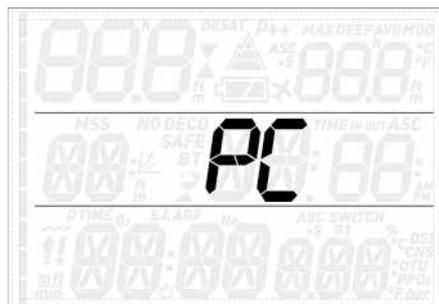
This submenu allows you to download your dive data to a PC or Mac. Press the **ENTER** button and the display will show **PC ready**, symbolizing that Quad is ready to communicate.
