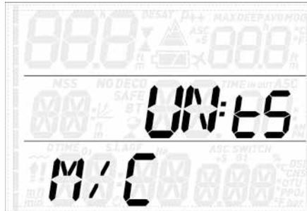
You can choose between metric (depth in meters, temperature in °C) and imperial units (depth in feet, temperature in °F).
