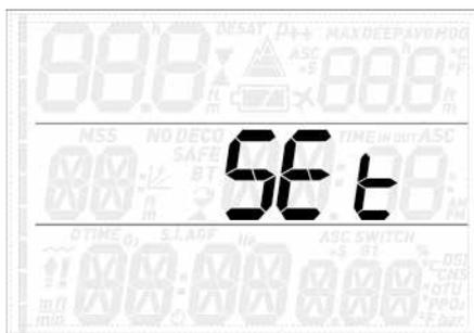
Quad's **SEt** menu allows you to change settings. Once inside this menu, press the **UP** or **DOWN** button to scroll between two submenus: **SEt dIVE**, where you can set parameters pertaining to the dive, and **SEt tIME**, where you can set parameters pertaining to time and date.
