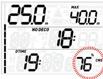
When the oxygen toxicity level approaches 100% the alarm is repeated for 5 seconds in one-minute intervals after the first occurrence and for as long as the value of CNS stays at or above 100%. Consider terminating the dive immediately!
