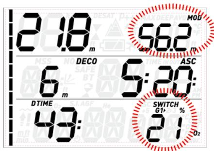
Press either of the lower buttons while this indication is blinking to initiate the gas switch: the oxygen percentage of G2 starts to blink in lieu of that of G1, and in the top right corner the MOD of G2 is displayed, also blinking.
