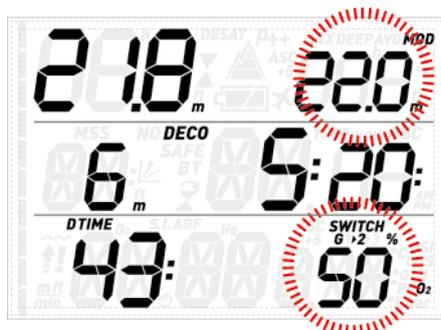
Press and hold either of the lower buttons to confirm the switch to G2: the set oxygen concentration will be displayed steadily in the lower right corner of the screen, and within 20 seconds the ascent time is updated to reflect the higher oxygen concentration in the breathing gas.
