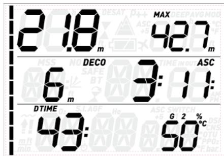
If you press either of the lower buttons while G2 is blinking, the next available gas in the list will be displayed instead. This will be G1 if only two gases are set or if you are deeper than the MOD of G3, or G3 if you have set three gases and are shallower than the MOD of G3.
