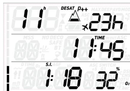
The other contains a condensed log of the last dive: maximum and average depth in the top row, dive time and set **O2%** in the bottom row. In addition, the bar graph shows the calculated nitrogen load in the leading tissue. You can use this to gauge your progress in getting rid of nitrogen as the surface interval grows. Quad continues to perform decompression-related calculations (nitrogen release), for as long as there is desaturation time left.
