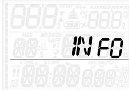
This submenu provides information about the hardware and software of your Quad and about the status of the battery: **OK** means the battery is good, **LOW** means the battery is weak but you can still do a few more dives, and **KO** means the battery is very low and Quad won't function as a dive computer.
