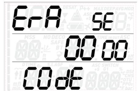
Quad allows you to reset the desaturation in the computer. Any tissue saturation information from a recent dive will be reset to zero and the computer treats the next dive as a non-repetitive dive. This is useful when the computer is loaned to another diver who has not dived in the last 24 hours.
