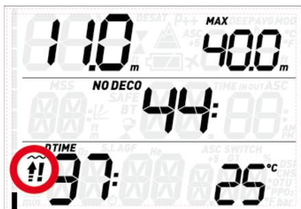
In this case, if the diver attempts a repetitive dive after surfacing, Quad will only function as a depth gauge and timer (bottom timer mode), and will display on the screen throughout the dive.
