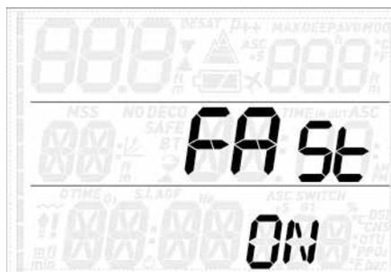
A fast (uncontrolled) ascent is defined as one in which a speed of 12 m/min / 40ft/min or higher was maintained over more than two thirds of the way up. This applies to dives deeper than 12m/40ft only. In such an event, due to the potential of harmful bubble formation, Quad locks the computer for 24 hours in order to discourage you from diving again. In this menu, you have the option to disable the locking up of the computer in the event of an uncontrolled ascent.
