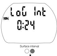
If there was a remaining desaturation time (DESAT) before selecting the logbook, the time since the last dive (surface interval) is displayed.
