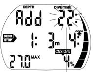
Set desired bottom time with  $\bigcirc$   $\bigcirc$  and  $\bigcirc$   $\bigcirc$
