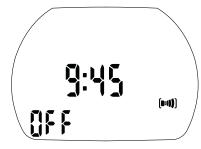
The alarm clock goes off only at the surface. "Sound" must be turned "on" in "set 2".
