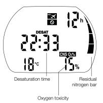
To check the elapsed surface interval press  $\bigcirc$   $\mathbb{O}$ .
