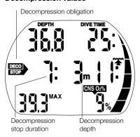
On entering the decompression phase, "NO STOP" disappears, the symbol appears and an attention beep goes off. The nitrogen loading bar stops flashing and the 6<sup>th</sup> segment lights up (red area). The deepest decompression stage in metres (feet) is displayed and the decompression
