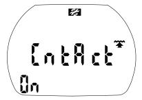
On submerging in water the water contacts switch on Aladin 2G automatically.
