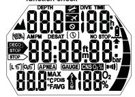
Switch on Aladin 2G by pushing  $\bullet$   $\circ$  and check the test display: Are all elements of the display activated? Do not use Aladin 2G if the display does not show all elements. When switching on Aladin 2G with  $\circ$   $\bullet$ , the test display will not appear.
