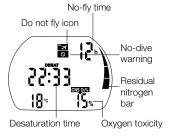
From the **time of day display** you can check the desaturation time\* by pushing  $\bigcirc$  • Desaturation time is determined either by oxygen toxicity, nitrogen saturation or the regression of microbubbles, depending on which requires the longer time.
