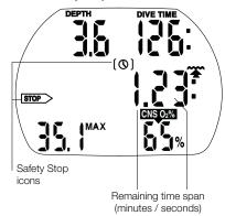
The safety stop timer displays the time span a diver should spend at the safety stop depth at the end of the dive. The timer starts automatically when depth is shallower than 6.5 m and counts back from 3 minutes (default) to zero. It can be restarted manually any number of times. The duration of the timer can be set between 1 and 5 minutes.
