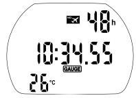
Remaining time during which Aladin 2G cannot be used in computer mode
