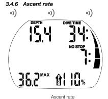
Optimal ascent rate varies depending on depth between 7 and 20m/min (23 and 67ft/min). It is displayed as a percent of the reference variable ascent rate. If the ascent rate is greater than 100% of the set value, the black arrow "SLOW" appears. If the ascent rate exceeds 140%, the arrow starts flashing.
