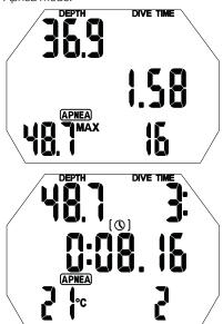
In Apnea mode the dive can be started manually by pressing ○ ●. This function allows fast sampling to start straight from the surface. Automatic start of the apnea dive will happen from depth of 0.8m/3ft. Once activated the Apnea mode will run 15 minutes after surfacing. This allows you to start a repetitive apnea dive with precise data in the logbook. Surface mode can be stopped with long press ○ ●.
