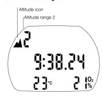
Aladin 2G measures the atmospheric pressure every 60 seconds even while the display is switched off. If the computer detects a sufficient increase in altitude, it switches on automatically and indicates the new altitude range (1-4) and the desaturation time. Desaturation time indicated at this moment refers to adaptation time at this altitude. If the dive starts within this adaptation time, Aladin 2G treats it as a repetitive dive, since the body is offgassing.
