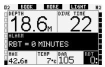
In **LIGHT** configuration, the alarm message **RBT** = **0 MIN** is displayed in place of the no-stop information for 12 seconds and during this time the audible signal goes off. In addition, after the text message extinguishes, the RBT is displayed in inverted colors (white on a black background) in the lower right corner. The audible signal does not stop unless the RBT grows to 1 minute or more, or if the depth is 6.5m/20ft or shallower.
