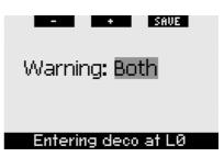
During the dive, if you are about to enter decompression and the warning is set to either **VISUAL** or **BOTH**, Galileo will show the message **ENTERING DECO AT L0** on the display for 12 seconds. The following figures show the actual display in the **CLASSIC** and **FULL** configurations.
