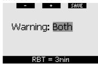
During the dive, if the RBT drops down to 3 minutes and the warning is set to either **VISUAL** or **BOTH**, Galileo will show the message **RBT** = **3 MIN** on the display for
