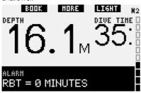
In **FULL** configuration, the alarm message **RBT** = **0 MIN** is displayed in place of the no-stop or decompression information for 12 seconds and during this time the audible signal goes off. In addition, the RBT information is displayed in inverted colors (white on a black background). The audible signal does not stop unless the RBT grows to 1 minute or more, or if the depth is 6.5m/20ft or shallower.
