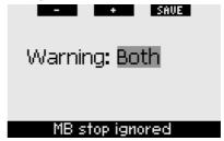
During the dive, if you ascend shallower than a suggested MB stop depth and the warning is set to either VISUAL or BOTH, Galileo will show the message MB STOP IGNORED on the display for 12 seconds and the depth is shown in inverted colors
