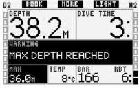
For the LIGHT configuration, the current depth is displayed in inverted colors (white on a black background) and will remain so until the diver ascends above the set depth.
