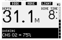
For the **FULL** configuration, the CNS O<sub>2</sub> is shown in inverted colors (white on a black background). This will remain so for as long as the CNS O<sub>2</sub> value is higher than 75%.
