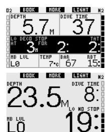
For **FULL** layout, the underlying L0 information is shown in the sequence right after the **BUDDY** tank pressure and before the ppO<sub>2</sub>. This is displayed instead of the MB level no-stop or decompression information and remains there only for 5 seconds, after which it is replaced again by the information relative to the active MB level.
