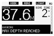
For the FULL configuration, the value of the set depth replaces the max depth indication and is shown in inverted colors (white on a black background). This will remain so until the diver ascends above the set depth.
