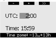
The range of the UTC setting is between 13 hours and +13 hours in 15 minute increments.
