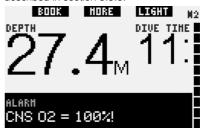
In **FULL** configuration, the alarm message **CNS O**<sub>2</sub> = **100%** is displayed in place of the no-stop or decompression information for 12 seconds and during this time the audible signal goes off. In addition, the CNS O<sub>2</sub> information is displayed in inverted colors (white on a black background) and remains displayed until the CNS O<sub>2</sub> value drops under 100%.
