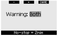
During the dive, if the no-stop time reaches 2 minutes and the warning is set to either VISUAL or BOTH, Galileo will show the message NO STOP = 2 minutes on the display for 12 seconds. The following figures show the actual display in the various dive configurations (CLASSIC, LIGHT and FULL).
