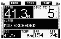
In **LIGHT** configuration, the alarm message **MOD EXCEEDED** is displayed in place of the no-stop information for 12 seconds, after which it is repeated in 4 second intervals. In addition, the current depth is displayed in inverted colors (white on a black background) and remains like this until the diver ascends 1m/3ft above the MOD. The audible signal persists until the diver ascends 1m/3ft above the MOD.
