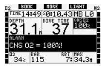
In all configurations, the alarm message and the audible signal are repeated for 5 seconds in 1 minute intervals after the first occurrence and for as long as the value of CNS  $O_2$  stays at or above 100% or until the pp $O_2$  drops under 0.5bar (see section 3.1 for a list of depths at which pp $O_2$  equals 0.5bar for some typical Nitrox mixes).
