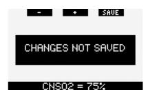
If more than one entity can be changed within a single menu, the right button is labeled ">>" instead of "SAVE". Pressing ">>" will move the highlighted segment to the next entity that can be changed. When the highlighted segment is on the last possible entity that can be changed, the right button reverts back to "SAVE". In case of submenus, the operation follows the same process.
