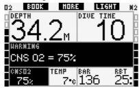
For the LIGHT configuration, after the text message extinguishes the CNS O<sub>2</sub> is displayed in inverted colors (white on a black background) in the lower left corner, alternating every 4 seconds with the tank pressure information. This will remain so for as long as the CNS O<sub>2</sub> value is higher than 75%. Alternate information is still available as described in section 3.3.3.
