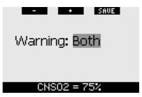
If a warning is set to **VISUAL** or **BOTH** and it is triggered while Galileo is in compass mode, the display will automatically switch back to the regular configuration (**CLASSIC**, **LIGHT** or **FULL**) in order to properly show the warning message.
