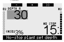
At any point, **press** ">>" to switch to the decompression dive planner for the indicated depth. Galileo will add 1 minute to the no-stop time and show the resulting decompression obligation.
