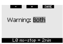
During the dive, if the underlying L0 no-stop time reaches 2 minutes and the warning is set to either **VISUAL** or **BOTH**, Galileo will show the message **L0 NO-STOP** = **2 MIN** on the display for 12 seconds. The following figures show the actual display in the **CLASSIC** and **FULL** configurations.
