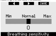
The sensitivity of the workload calculation to changes in breathing pattern can be adjusted in 25 steps: this has an effect on how the algorithm accounts for changes in breathing pattern in the decompression calculation.
