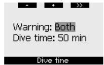
During the dive, if the dive time reaches half the value of the set dive time and the warning is set to either **VISUAL** or **BOTH**, Galileo will show the message **TURN-AROUND TIME** on the display for 12 seconds. The following figures show the actual display in the various dive configurations (**CLASSIC**, **LIGHT** and **FULL**).
