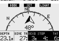
In this lay-out, the button functions change slightly. The middle button is now marked "SET". Pressing this button will set the bearing. Compass bearing represents the direction the front of the computer is pointed at. It is expressed in degrees, from 0 to 359. 0 degrees is North, 90 degrees is East, 180 degrees is South, 270 degrees is West and any other reading is interpolated in between.
