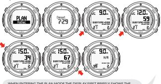
WHEN ENTERING THE PLAN MODE THE DISPLAY FIRST BRIEFLY SHOWS THE REMAINING DESATURATION TIME BEFORE GOING INTO PLAN MODE. USE UP AND DOWN BUTTONS TO SCROLL NO-DECOMPRESSION LIMITS AT DIFFERENT DEPTHS. YOU CAN ALSO ADJUST YOUR SURFACE INTERVAL TIME TO YOUR PLAN. NO-DECOMPRESSION LIMITS LONGER THAN 99 MINUTES ARE DISPLAYED AS "-"
