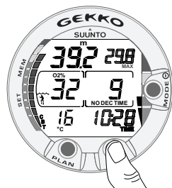
Fig. 3.24. Alternative display. Pressing TIME button displays current time, maximum depth, temperature, CBT and O_2\% ,
