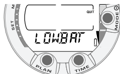
Fig. 3.2. Startup II. Battery power indicator.
