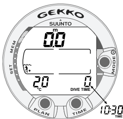
Fig 3.3. Startup III. Surface mode. Depth and dive time are zero, current temperature, 20 °C. Pressing TIME button activates alternative display of current time.
