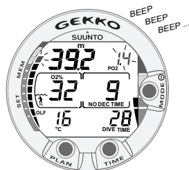
Fig. 3.23. Oxygen partial pressure and OLF displays. There is an audible alarm as oxygen partial pressure is greater than 1.4 bar or set value, and/or the OLF has reached 80% limit.
