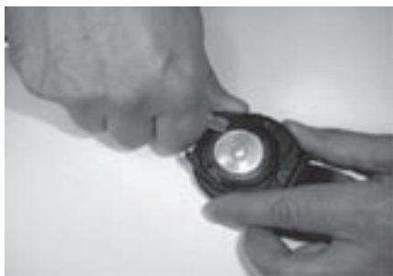
Fig. 5.2 Opening of the securing ring.
