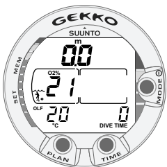
Fig. 3.21. Surface display in the Nitrox mode
