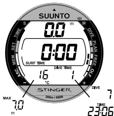
Fig. 3.32. Surface display after Free dive. Center window showing surface time.
