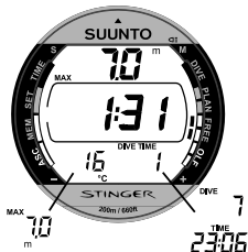
Fig. 3.33. Alternating surface display after Free dive. Center window showing the dive time of the most recent dive.
