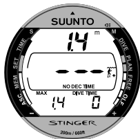
Fig. 3.10. Dive has just begun. Available no-decompression time is more than 199 min.
