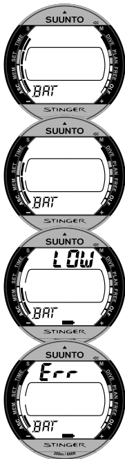
Fig. 3.3. Startup II. Battery power indicator.
