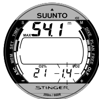
Fig. 4.9. Setting Oxygen Percentage and Partial Pressure.
