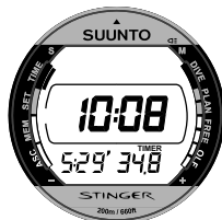
Fig. 2.7. The Stopwatch displays hours, minutes and seconds.
