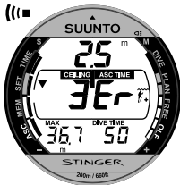
Fig. 3.20. Decompression dive, above ceiling. Note downward pointing arrow, Er warning and an audible alarm. You should immediately (within 3 minutes) descend to or below ceiling.
