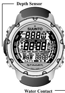
Fig. 2.2. The water contact and depth sensor.
