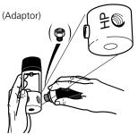
Fit the transmitter to the HP outlet. If the threads do not match, get an adaptor from your diving retailer.
