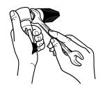
Tighten the transmitter by means of a size 19 wrench.
