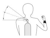
Position of the transmitter for righthanders, if there is no connection possible on the right hand side.
