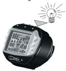
The display of TEC can be illuminated both on the surface and underwater.
