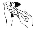
Tighten the transmitter by means of a size 3/4" wrench.
