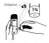
Mount the transmitter at the HP oulet. If the threads do not match, you can get a fitting adaptor at your diving equipment retailer.
