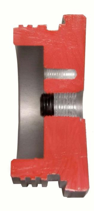
You will now be assembling the hose to the Light Head and the metal Canister End Cap. Before you start, apply a small amount of grease to the *Light Head* and *End Cap O*-*Ring* seating areas. These areas are where Hose O-Rings will seal. Lubricate both hose O-Rings, and then apply a small amount of Loctite #242 Blue (thread-locking fluid) to the threads. Do not get any on the *O-Rings*! (If you do, replace the O-Ring) and repeat the previous steps.
