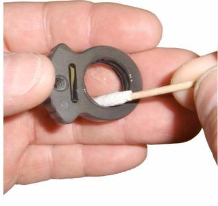
Place the flat washer over the hose support standoff, and apply grease to the washer.
