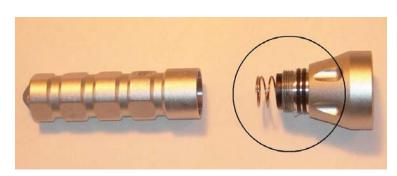
**Required Maintenance:** Apply an anti-seize compound to the threads of the flashlight head then apply silicone lubricant to the threads and O-Rings. Apply a minimal amount barely visible. Threads must be wiped off with a lint-free cloth and anti-seize compound must be applied at least every 2 months. More frequent maintenance may be required under harsh conditions or heavy use.
