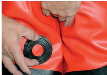
Attach the Pee Valve into the Valve Port with the socket of the attachment nut pointing upwards.
