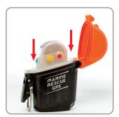
Unscrew two screws on top cap
