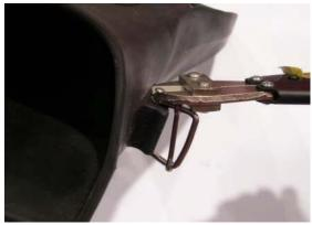
2. Cleanly cut the head of the buckle pin with bolt cutters or end cutter. Do not pull or twist the buckle pin.
