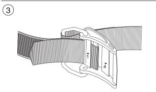
At this point stretch firmly in the indicated direction, so to let the belt firmly adhere to the tank.
