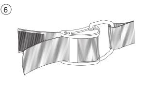
The buckle will close with a sharp click, blocking the back-pack on the tank.
