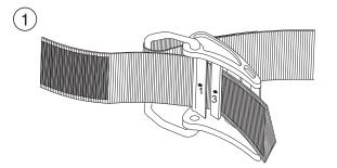
Following the arrow (1) insert the extremity of the belt from the inner side towards the external part of the buckle (between the sewn stirrup and the moving part) From the external side follow the arrow and go back to the inner side between the arrows (3 and 4).
