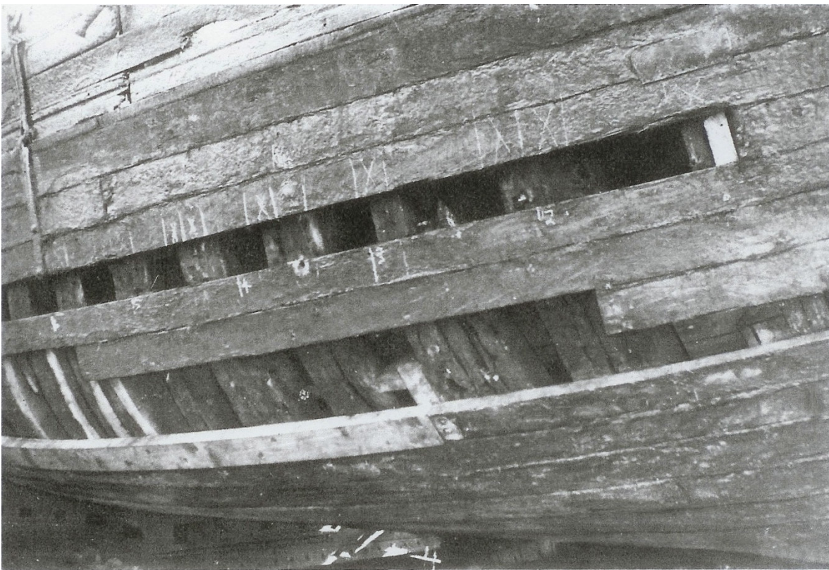
Fig. 3. The carvel construction of a wooden ship under repair, with its planks attached edge-to-edge to the ribs (17).
